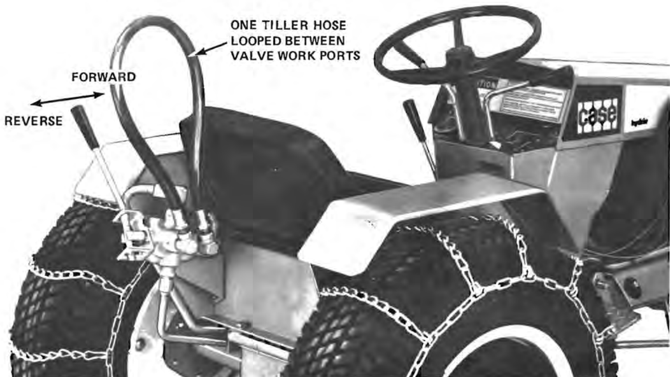
FIGURE 1 Model 444 Tractor With Hydraulic PTO Attached
