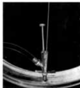
Tire rotated so valve is at bottom with hydroinflation fluid being removed.
